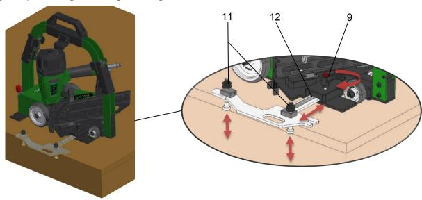
Proceed as follows for operation with the built-in parallel guide (12) on the edge of a panel or using the guide sight slot (19) on a specified line:
