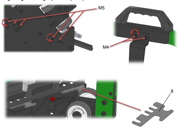
You can adjust the driving depth of the fasteners in the material by inserting or removing spacer plates in different positions. Six spacer plates, each 1 mm thick, are included in the delivery. When fitted, each spacer plate increases the opening distance to the material by 1 mm.
