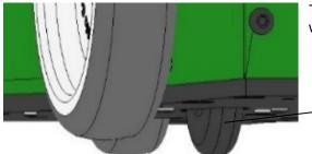
The Slider is equipped with a safety castor (17) underneath which only allows triggering when the tool is set down.
